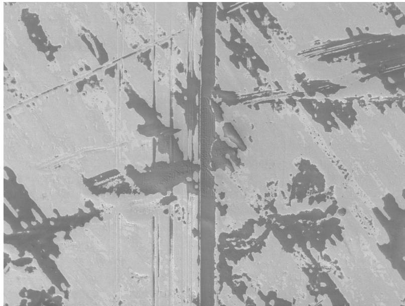
Fig. 3: Copper plate after 240s plasma treatment (200x magnification)
