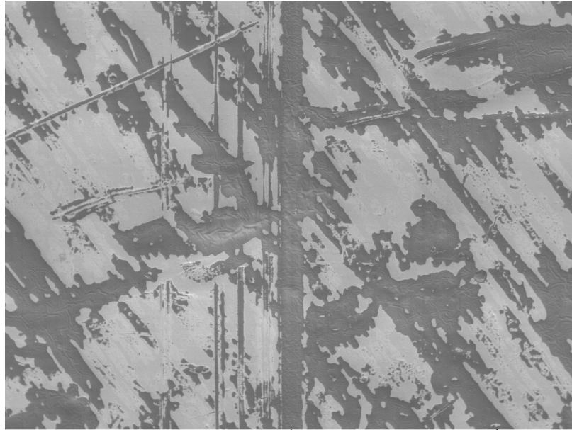
Fig. 2: Copper plate after 120s plasma treatment (200x magnification)
