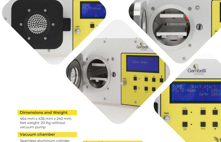
Seamless aluminum cylinder with a volume of 2 L (128.6 in<sup>3</sup>) - Ø 102 mm W 256 mm, with black anodized aluminum hinged door with screened visual specula.
